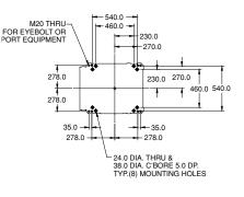
Note: Dimensions are shown in millimeters. Detailed CAD data are available upon request.
